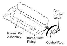
Figure 10 - Installing Gas Control Valve
